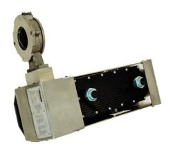
The AVB3.0 all-electric bleed air valve controls high-temperature air maintaining a precise fuel-to-air ratio within the turbine, facilitating optimal engine efficiency and meeting today's stringent emission requirements. Each valve incorporates a fail-safe spring configurable to fail open or fail close, depending upon the desired action. The AVB3.0 actuation mechanism has a unique torque shaft design, eliminating actuator side loading.
